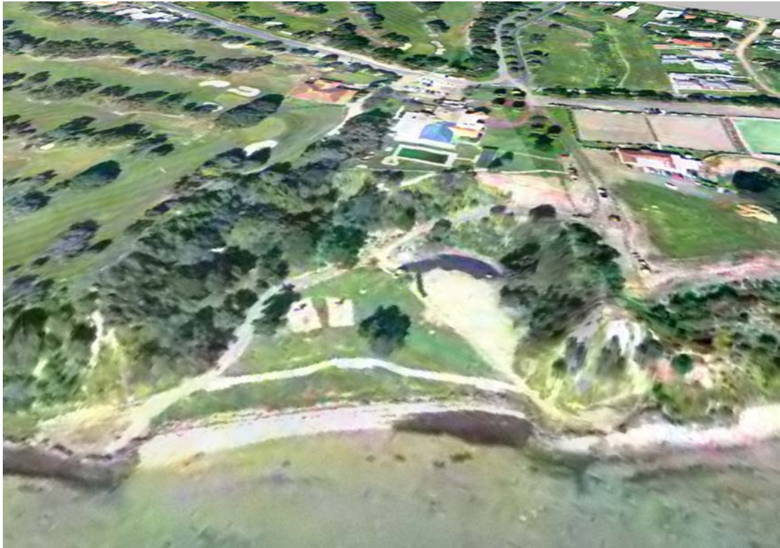
Figure 12. Oblique view of orthophoto imagery draped over terrain model (looking from Azimuth 330°, inclination 35°, distance 300 m. No vertical exaggeration)
