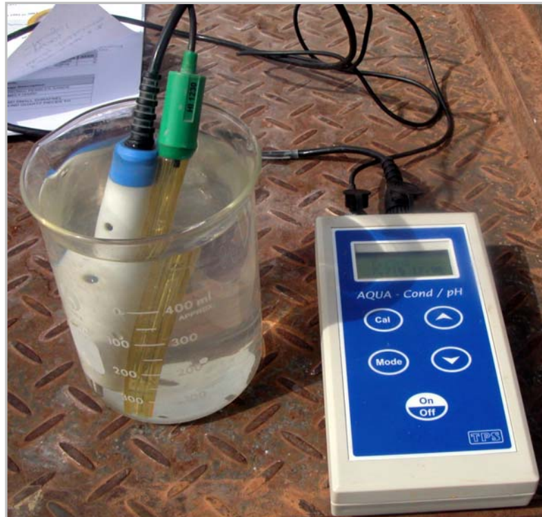
Figure 4.3 Aqua TPS Conductivity/pH meter with probes immersed in a beaker filled with sample water
