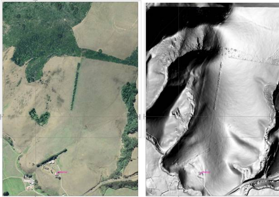
Figure 6 Tree artifacts in a 1.0m DEM near Johanna, Otway Ranges, Victoria, Australia
