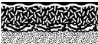
ORGANIC CHIP MULCH, 10-15CM THICK DEAD WEEDS (E.G. VIA HERBICIDE APPLICATION) SOIL
